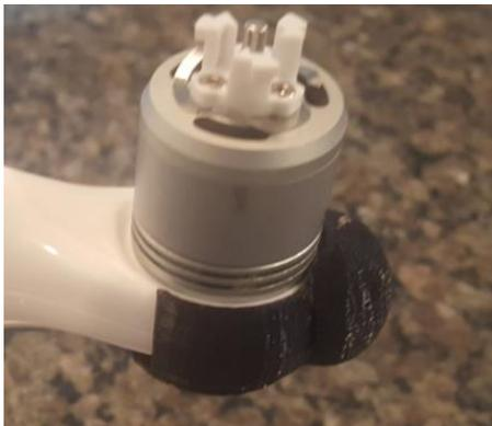
The rounded piece at the end of the holder is designed to keep the sun light away from the sensor. The holder is designed to not block the motor or the venting.
